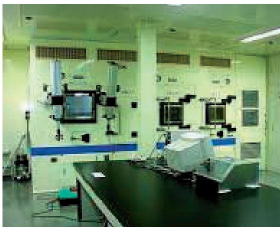
FIG. 9. Typical PET hot cell.
