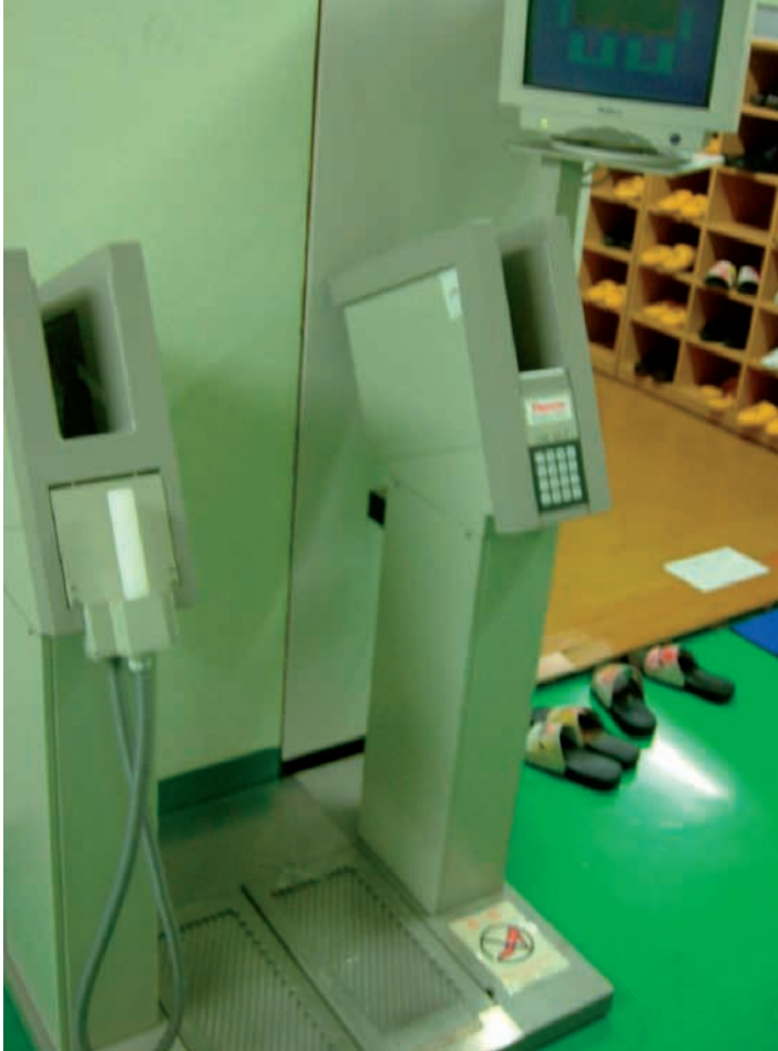
FIG. 4. Hand and feet contamination monitor.
